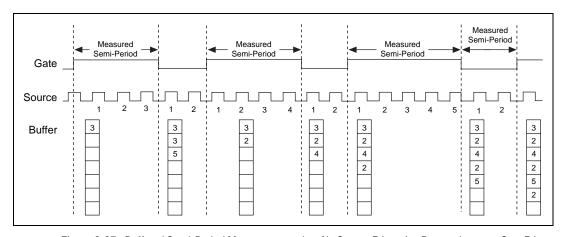
Figure 2-27. Buffered Semi-Period Measurement when No Source Edges Are Present between Gate Edges
